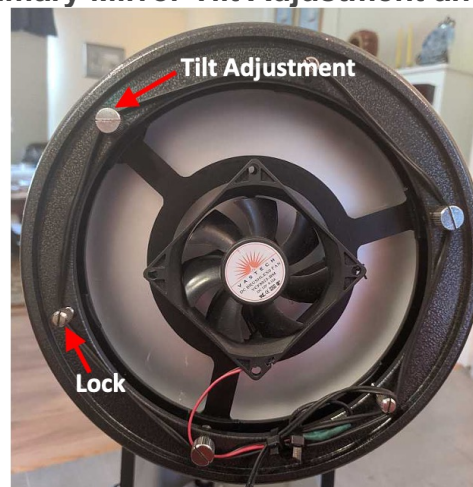
Figure 12: Primary Mirror Tilt Adjustment and Lock Screws
