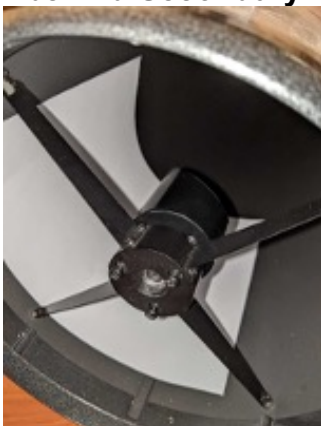
Figure 2a: White sheet inserted behind Secondary
